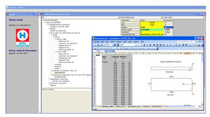
QTRANS can calculate transport motions and accelerations by either Noble Denton (interface with an inhouse spreadsheet) or Seakeeping analyses program Moses ( <u>satellite</u> program). Further the structural general and local strength of the cargo and barge is calculated with the integrated programs SACS and ROARK respectively. These are from importance for the grillage and seafastening design at the barge.
