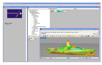
DESIS 3.0 uses Marin's DESP for speed power predictions (see also QDESP). An extensive mass calculation based on the SWBS (Ship Work Breakdown Structure) is included. Hydrostatics an the first indication of the intact stability performance of the concept design is determined by Rhinomarine (plug in of Rhinoceros).
