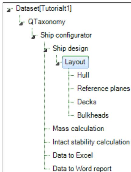
A ship design always contains a layout with at least a hull and defined reference planes. The entities *Decks* and *Bulkheads* will be optional for a user to include in their ship design.
