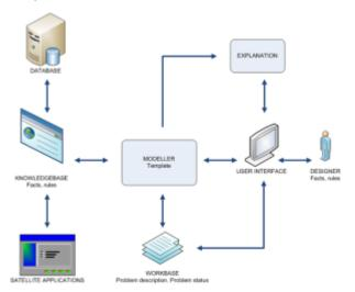
The combination of a project (a project file), a knowledge base (a knowledge file) and the Quaestor program makes a knowledge-based system to streamline design and engineering processes (workflows).
