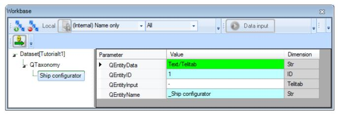
Every entity automatically contains the standard Quaestor parameters: *QEntityName* and *QEntityID*. Both parameters will not be visible during a process dialog for users. The value for *QEntityID* is unique and is automatically assigned by Quaestor. It cannot be modified by a Knowledge Engineer.
