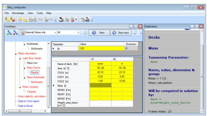
Again, a yellow cell means that a value is be determined by a relation. The parameters Nr, Name of deck, and Area are automatically copied from the defined Deck entities below Lay out. When you add or remove a deck, or change properties of an existing defined deck, these adaptations will be automatically propagated to the Mass Decks entity.
