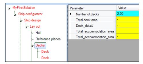
Next you have to define a name and a deck function for every deck. A deck function can be selected from a drop down box. To locate a deck within your ship design, you have to relate the aft and front position of a deck to one of your defined transverse reverences planes and the height of a deck to one of your defined horizontal reference planes. You can refer to your defined reference planes by selecting one of your defined reference names that will be shown in a drop down menu.
