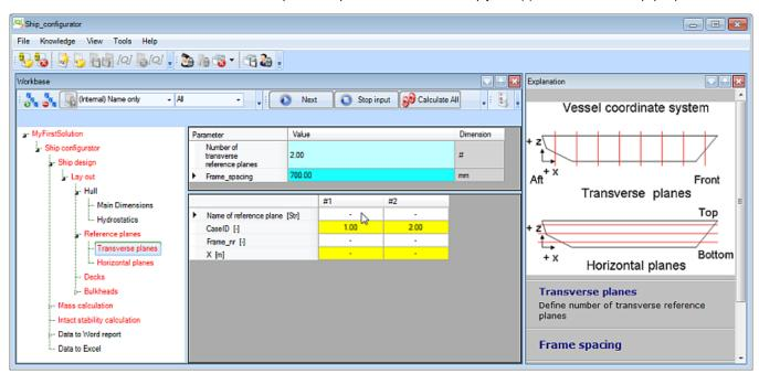
Now a table of 2 columns is created in the **table view**, each representing a transverse reference plane. You have to enter a frame number and a name for every plane (any recognizable name will do). Quaestor will calculate the X position of a transverse reference plane by X = Frame\_nr \*Frame\_spacing.
