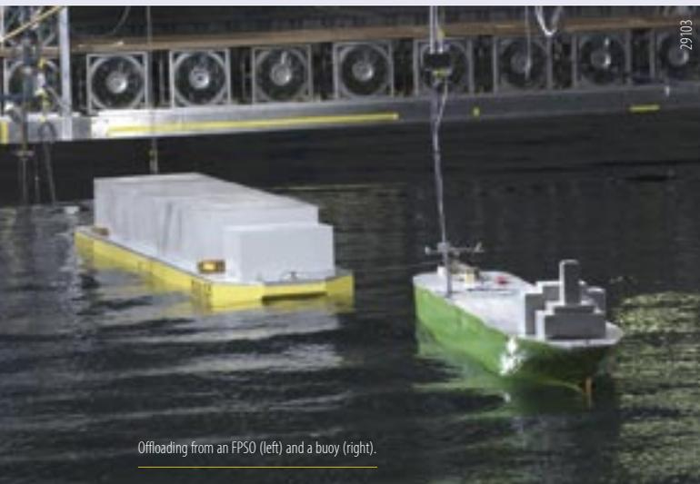
Offloading from an FPSO (left) and a buoy (right).
