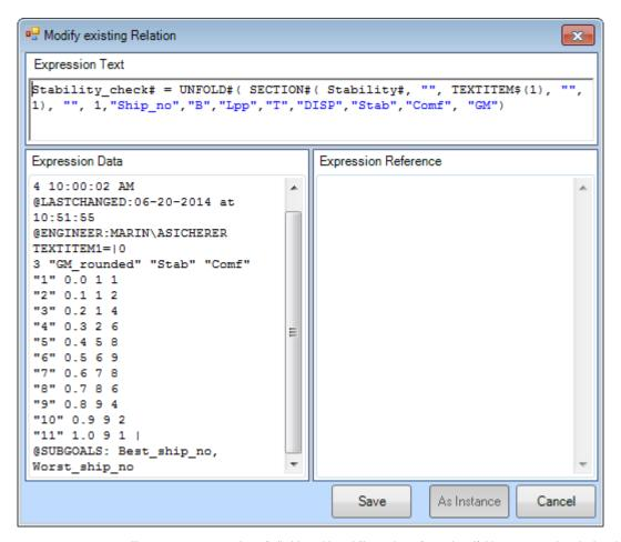
The parameter Stability\_check# will now return an overview of all ships with stability and comfort rating. If this parameter is calculated, the best and worst ship number will be added to the solution because of the attribute above.
