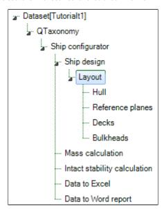
A ship design always contains a layout with at least a hull and defined reference planes. The entities <code>Decks</code> and <code>Bulkheads</code> will be optional for a user to include in their ship design.
