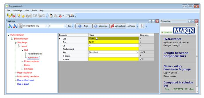
You see that yellow and white cells are shown. A yellow cell means that a value is a Top Goal for the analysis (inside the entity) and it will be determined by a relation. For example, select Lpp in the Entity (shown in Figure 13) and you can see that the value is computed by means of the relation Lpp = Entity#(20).Lpp, as shown in the **Explanation window** on the right.
