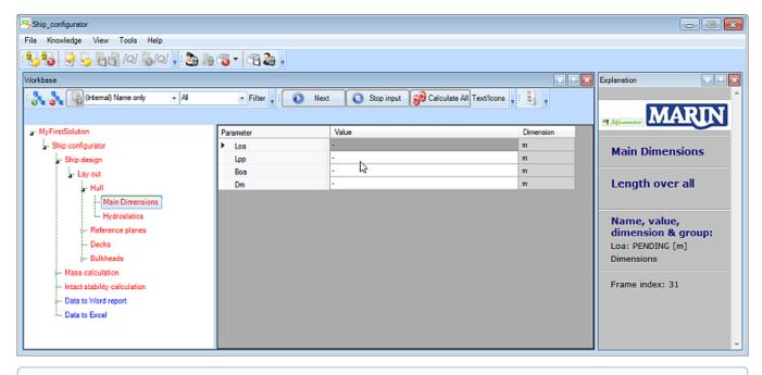
A white cell means that input values from the user are needed.
