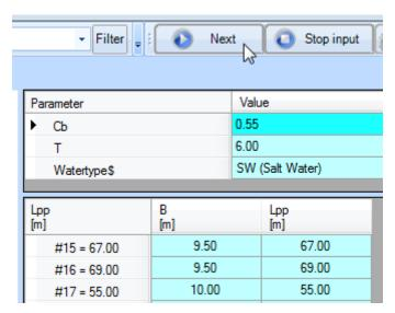
The new solution is now created. The fixed values are again shown in the right hand side of the workbase. The varying parameters (B and Lpp) and the corresponding solution for DISP are shown in the lower part. Each row is a different **case**, identified by a **case number**(#1, #2, etc.).
